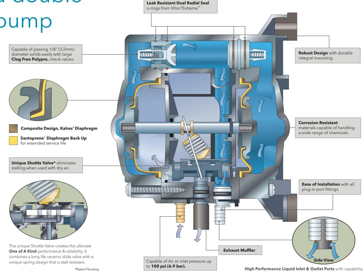
of supplying flow rate to 5 GPM (18.9 l/min.).
