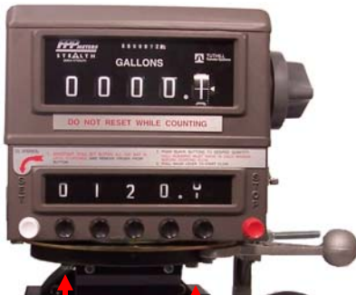
Register stack attaches to the RAD with 4 screws, 2 front and 2 rear.
