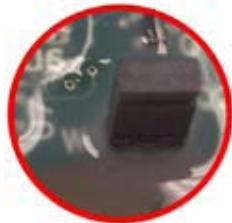
Both pins covered: 5VDC Regulated = EL0300-5-1
