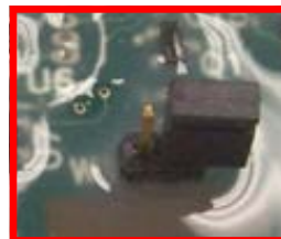
1 pin exposed: 5.5 - 12 VDC = EL0300-5-3
