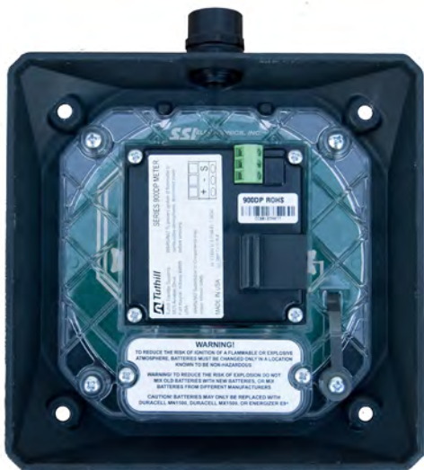
900DP Battery and Wiring Access
