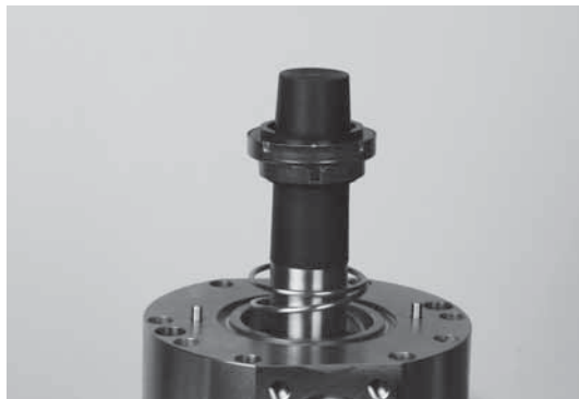
36. Mount shaft seal in flange
