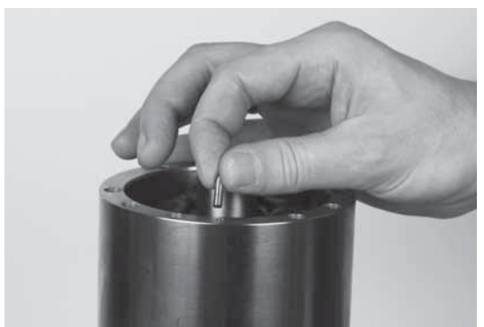
24. Mount 1 guide pin in pump housing
