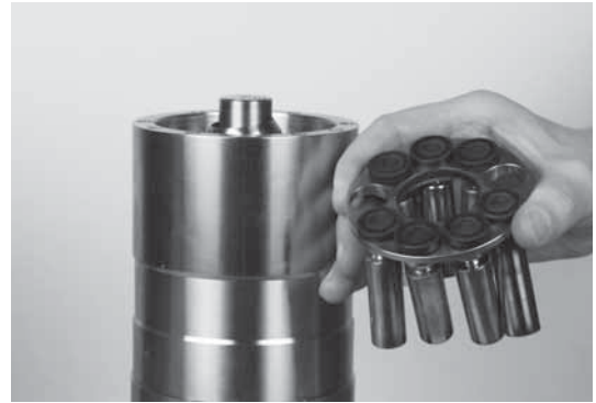
22. Mount pistons in housing
