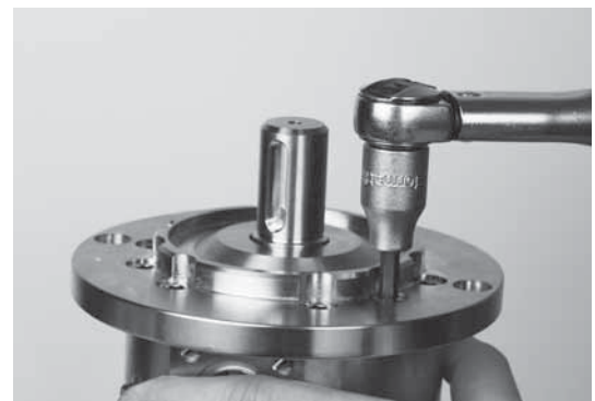
40. Tighten with 30 Nm
