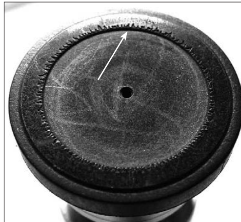
Picture 3: Cavitation of the piston shoes. All pistons must be replaced within the next 100-200 hours.
