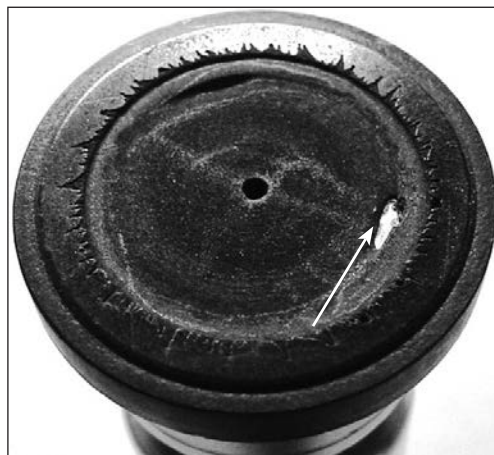
Picture 3: Cavitation of the piston shoes. All pistons must be replaced within the next 100-200 hours.
