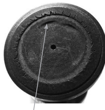
Cavitation of the piston shoes. All pistons must be replaced within the next 500-1,000 hours.
