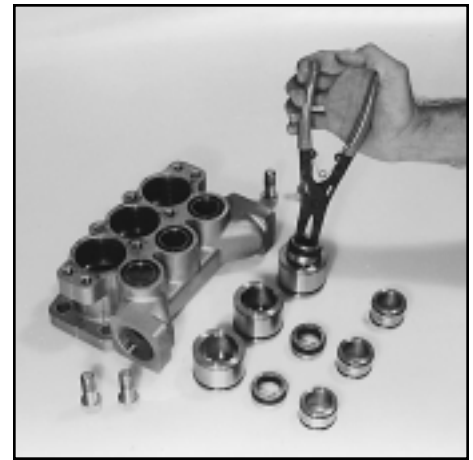
Removing the Female Adapter, V-Packing and Male Adapter
