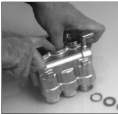
Installation of Male Adapter
