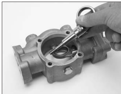
6.8 Install plunger rod/connecting rod assembly through large opening in crankcase body (1).
