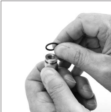
6.13 Lubricate and install o-ring (23) to seat (24). Repeat for second valve assembly.
