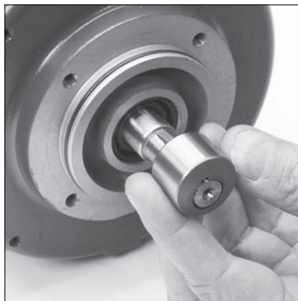
5.5 Remove and inspect cam (8) from motor shaft.
