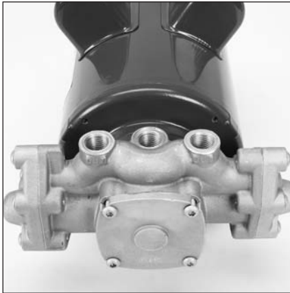
1.6 Pump inlet port facing motor.
