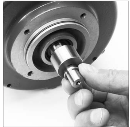
6.6 Install retaining ring (7) into snap ring groove on motor shaft to secure cam (8).
