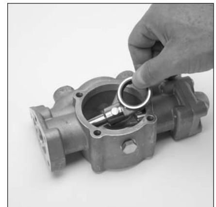
5.15 Remove and inspect connecting rod, plunger rod and wrist pin assembly.
