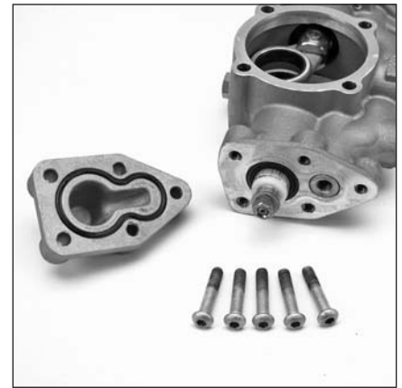
5.9 Remove five (5) M6x30 screws (13) holding head cover (14) to crankcase body.
