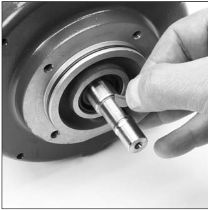
6.4 Lubricate and install woodruff key (9) into motor shaft keyway.
