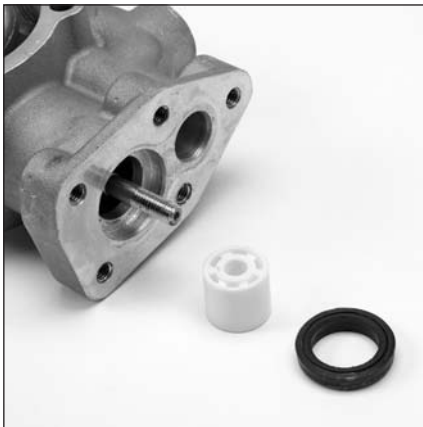
5.14 Remove and inspect ceramic plunger (21) and high pressure seal (22) from crankcase body (1).
