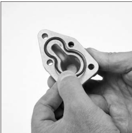
6.22 Lubricate and install o-ring (15) into head cover. Repeat for other cylinder head.
