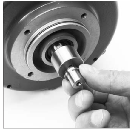
6.6 Install retaining ring (7) into snap ring groove on motor shaft to secure cam (8).
