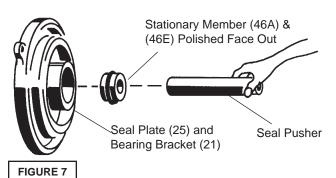
Make sure the stationary members are in straight and that the rubber ring is not out of it's groove. Slide a bullet (see parts list-Seal Kit) over motor shaft. Lightly oil (DO NOT use grease) shaft, bullet and inner surface of bellows on rotating member (46D) see Figure 8. With lapped surface facing bearing bracket (21), slide rotating member (46D) over bullet and onto shaft, using seal pusher, until lapped faces of (46D) and (46E) are together (see Figure 6).
