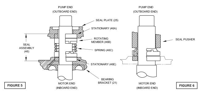
**Seal -** Clean and oil seal cavities in bearing bracket (21) and seal plate (25). Lightly oil **(DO NOT use grease)** outer surface of inboard stationary member (46E) and outboard stationary member (46A). Press inboard stationary member (46E) firmly into bearing bracket (21) and outboard stationary (46A) into seal plate (25), using a seal pusher (see parts list- seal tool kit), nothing but the seal pusher is to come in contact with seal face (See Figure 7).
