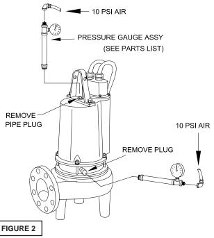
**Seal Chamber -** Remove pipe plug (22) from Bearing Bracket (21) and check that seal chamber is full of oil. Apply pipe sealant to pressure gauge assembly and tighten into hole in bearing bracket (21). Pressurize seal chamber to 10 PSI and check for leaks as outlined above.
