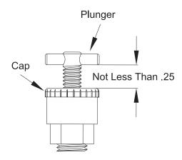
The plunger and handle should be no less than 1/4" above the cap which indicates the seal chamber is full or pressurized. If less than 1/4" above cap, the seal chamber needs additional lubricant.
