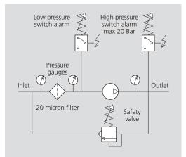
Solenoid valves should not be installed in the circuit; however, if needed, a mechanical safety valve needs to be installed before the solenoid valve, in order to protect the pump from pressure peaks.
