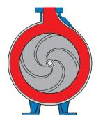
Both the modified concentric volute and partial splitter minimize radial loads and distribute pressure evenly across the entire flow range for less stress and wear on components. Casing meets ANSI B73.1 dimensional requirements for foot and flange.
