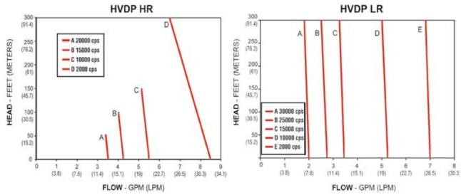
Flow rates are dependent on the properties of the fluid and its ability to flow freely into the pump intake. Expected flow rates for fluids above 30,000 cP are 1 to 3 gpm (3.8 to 11 lpm).
